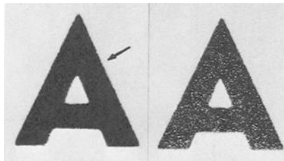
FIG. 7—Side-by-side comparison of two different photocopy processes: (left) lead edge of light passing over original to produce the copy and (right) the beaded appearance of the light reflecting off a copy. The beaded appearance is due to the heat-fusing of the toner to the copied page.
