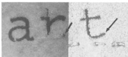
FIG. 3—Original document (left) and lift-off tape (right) typed on an IBM Correcting Selectric typewriter.
